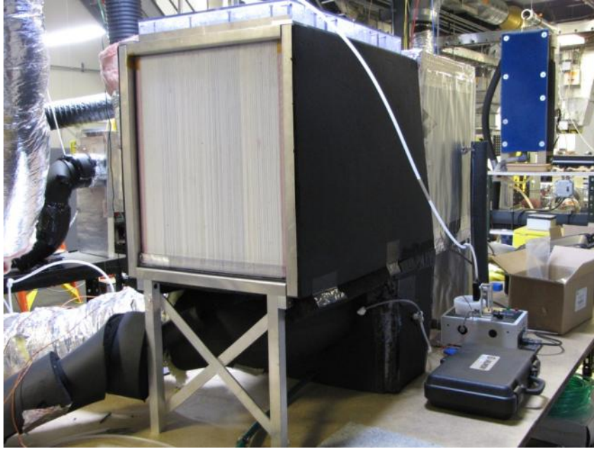
Figure 2–7 Fully assembled view of AIL Research second-stage conditioner (outlet airstream 2 shown)
